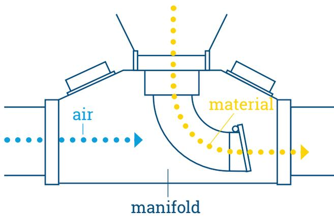
Mixing chamber for velocity-dependent systems
