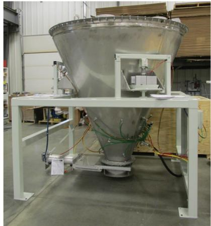
*Cyclonaire batch weigh hoppers are engineered with flexible isolation joints to minimize outside forces that can affect weighing.*
