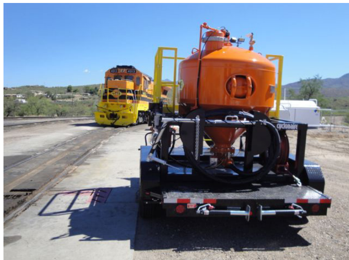
Cyclonaire's Sand-A-Long is an innovative sanding conveyor stationed on a trailer which allows a single operator to fill a locomotive's sanding box anywhere at any time.
