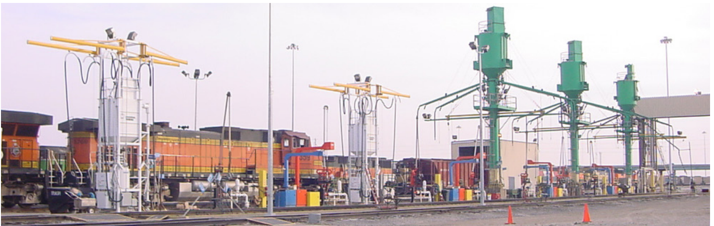
Cyclonaire's Mainliner System simultaneously services the fore and aft sandboxes of up to five locomotives on one track, or five locomotives on a parallel track.
